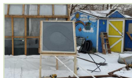
Our greenhouse Project Leader stays innovating, by designing and building this Solar Hot Water heater module to enable aquaponic operation during winter.
